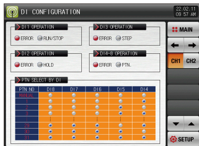
[Fig. 12-2] DI function and operation setting screen #2 (Channel 1)
