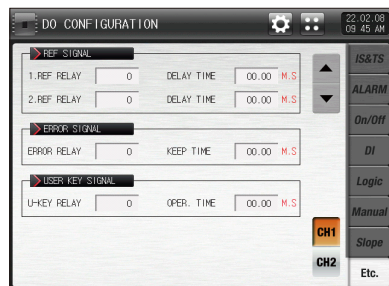
[Fig.11-10] Sub output relay setting screen #2
