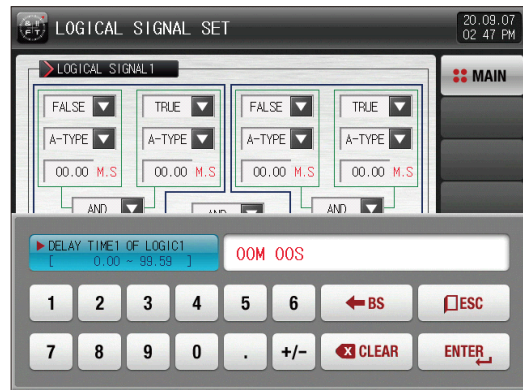
[Fig. 7-4] Logic signal delay time setting screen
