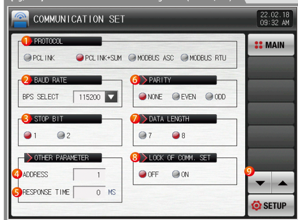
[Fig. 10-3] Communication environment setting screen (RS232C/485)
