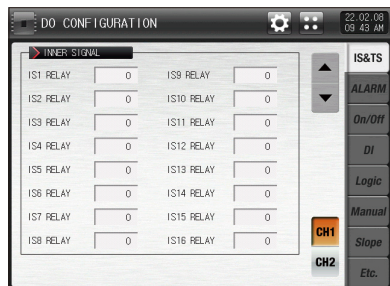
[Fig. 11-1] Inner signal relay setting screen #1
