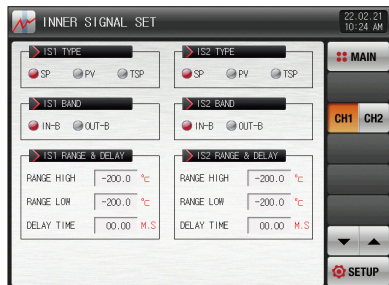
[Fig. 5-1] Inner signal setting screen #1 (Channel 1)
