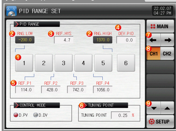
[Fig. 9-1] PID application range setting screen #1
