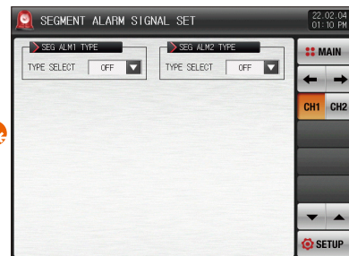
[Fig. 8-5] SEG alarm signal selection screen (Channel 1)
