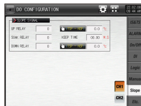
[Fig. 11-8] Up/soak/down signal relay setting screen
