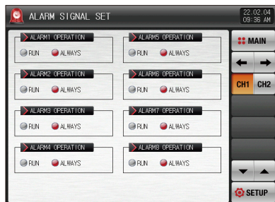
[Fig. 8-1] Alarm signal selection screen #1
