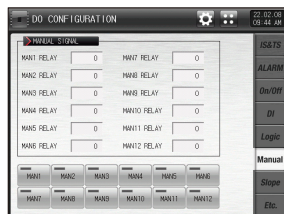
[Fig. 11-7] Manual signal relay setting screen
