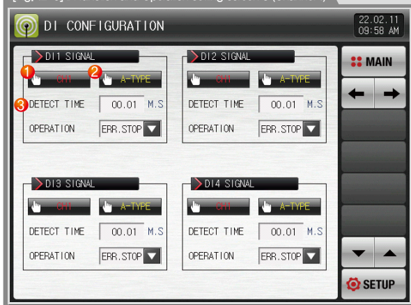
[Fig. 12-5] DI function and Operation setting screen 3 (Channel 1)
