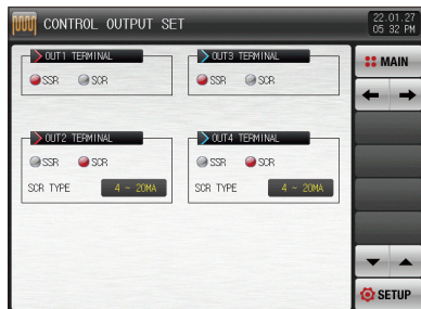
[Fig. 4-1] Output type selection screen (General)
