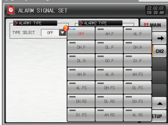
[Fig. 8-3] Alarm signal selection #2 in screen 2
