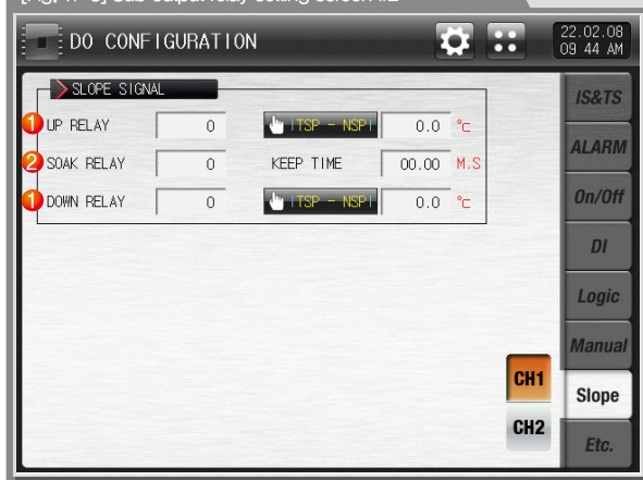
[Fig. 11-8] Sub output relay setting screen #2
