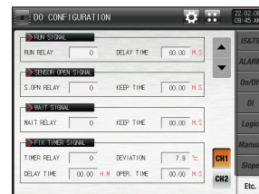
[Fig. 11-9] Sub output relay setting screen#1
