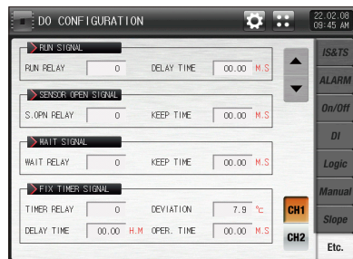
[Fig.11-9] Sub output relay setting screen #1
