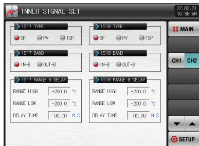
[Fig. 5-2] Inner signal setting screen #1 (Channel 2)
