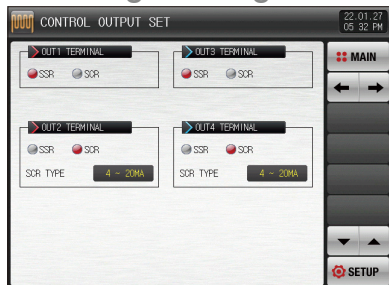
[Fig. 4-7] OUT output type selection screen (Heating · Cooling)
