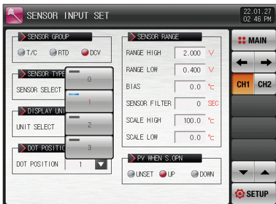
[Fig. 3-9] Screen for selecting the decimal point for the sensor
