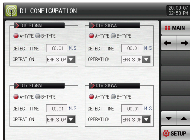
[Fig. 12-4] DI function and operation setting screen 2 #2
