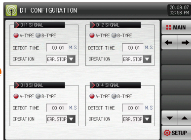
[Fig. 12-2] DI function and operation setting screen 2 #1
