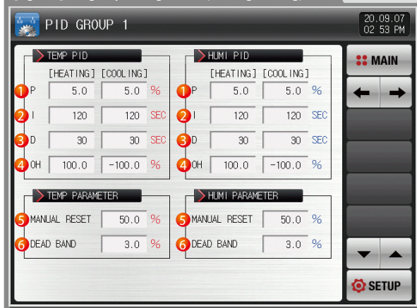
[Fig. 9-6] PID group setting screen (Heating-Cooling)
