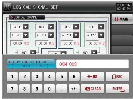
[Fig. 7-4] Logic signal delay time setting screen
