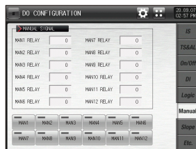
[Fig.11-7] Manual signal relay setting screen
