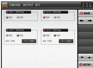
[Fig. 4-1] Output type selection screen (General)
