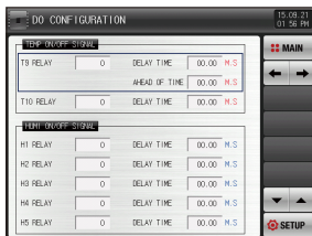
[Fig. 11-4] Humi ON/OFF signal relay setting screen
