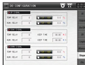
[Fig.11-8] Up/soak/down signal relay setting screen
