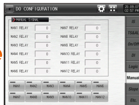
[Fig. 11-6] Manual signal relay setting screen
