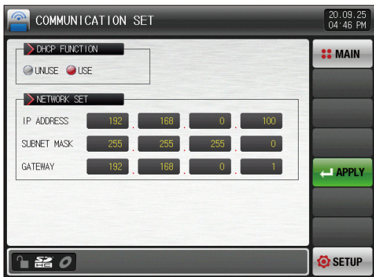
[Fig. 10-6] Ethernet DHCP use screen
