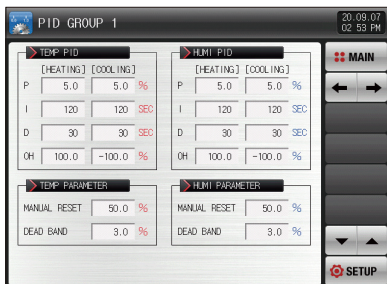
[Fig. 9-6] PID group setting screen (Heating-Cooling)
