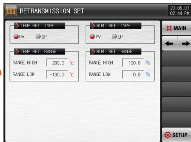
[Fig. 4-9] Transmitting output setting screen (In case of PV, SP setting)
