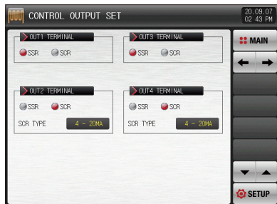
[Fig. 4-5] OUT output type selection screen (Heating-Cooling)
