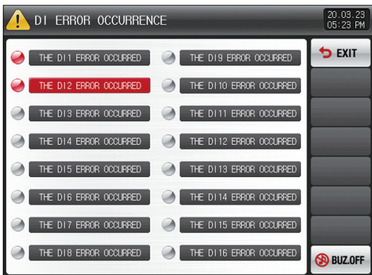
[Fig. 12-11] The screen with letter for DI error display method
