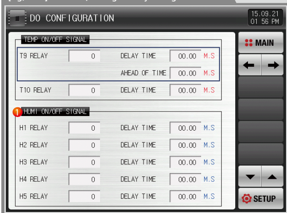
[Fig. 11-4] Humi ON/OFF signal relay setting screen
